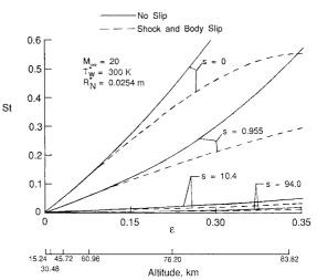
Fig. 4 Stanton number distribution for a 5-deg sphere cone from VSL method.
