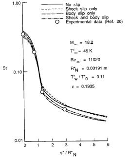
Fig. 2 Stanton number distribution for a 10-deg sphere cone from VSL method.
