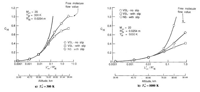
Fig. 7 Stagnation-point, heat-transfer coefficient vs Knudsen number and altitude.
