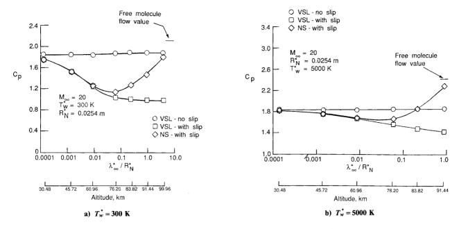
Fig. 6 Stagnation-point pressure coefficient vs Knudsen number and altitude.
