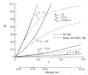
Fig. 5 Stanton number distribution for a 10-deg sphere cone from VSL method.
