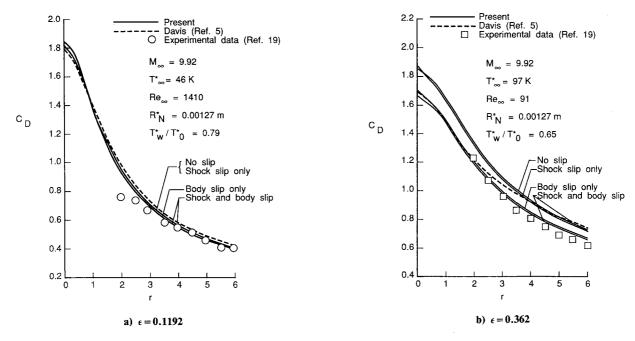
Fig. 1 Drag coefficient for a 10-deg hyperboloid from VSL method.
