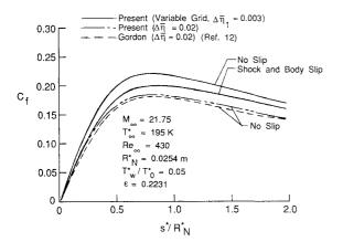
Fig. 3 Skin-friction coefficient distribution for a 22.5-deg hyperboloid from VSL method.
